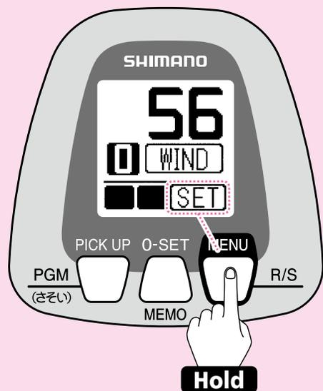
**4** After completely finishing winding on the backing line, press the 0 SET button for more than 3 seconds.
