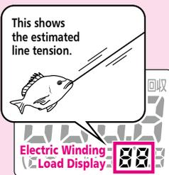
This shows the estimated line tension when the motor is winding up the line. Drag adjustment and winding speed adjustment can help prevent the leader from snapping, and are also factors in determining the size and number of fish that can be caught.
