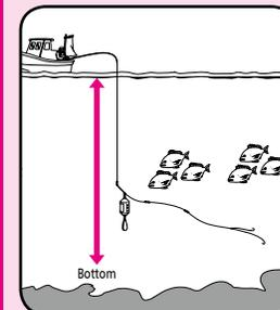
You can store the water depth from the surface or from the bottom, and display it in the Saved Depth column. In Bottom-Up mode, the depth is displayed in the Saved Depth column with the saved position represented by 0.
