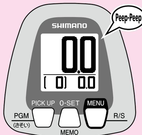
**1** If you break your line, after repairing it, lower your rig to the surface and press 0 Set for more than 3 seconds.
