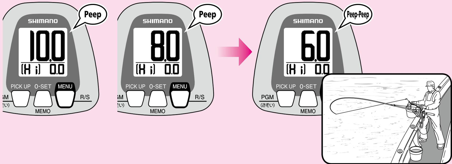
**1** 4m before the Gunwale Stop Position the alarm will sound every 2m. The diagram above shows the display when winding in using the Technical Lever in HI.
