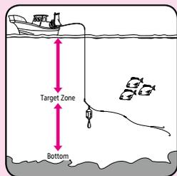
If you would like to check the depth from the bottom in accordance with the fishing location, fishing method and the type of fish being caught, you can change the saved depth display method. In Top-Down mode, the saved depth is displayed, but if you select Bottom-Up mode, you can check the depth with the saved depth position represented by 0.
