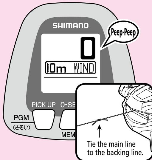
**5** The alarm will sound (peep-peep) and the display will appear as shown in the diagram. Once winding-on is finished, tie the main line to the backing line.
