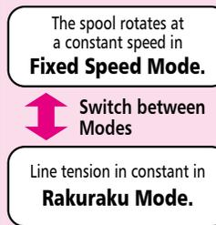
Change between Rakuraku Mode, which maintains a constant tension and prevent line slack, and Fixed Speed Mode, which maintains spool rotation at a constant speed.
