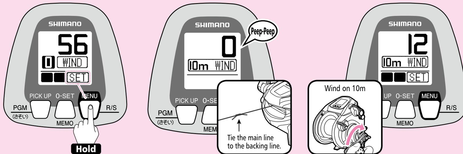
**4** After completely finishing winding on the backing line, press the MENU button for more than 3 seconds.
