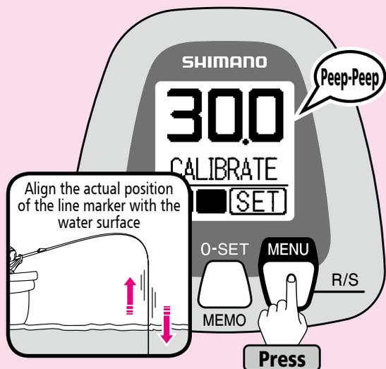
**3** Adjust the display to match the actual position of the line (30m in this example) on the surface of the water.
