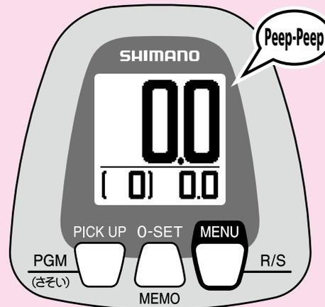
**1** Lower the rig to the surface and press 0 Set for more than 3 seconds.
