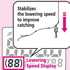
"( )" flashes while the estimated lowering speed is being displayed. Stabilising the lowering speed can assist with improving the success of hooking.
