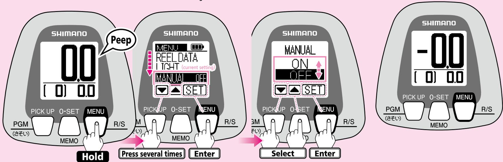
**1** When the power is turned on, Manual Mode is set to OFF. The illustration shows the Water Depth Display with Manual Mode OFF.
