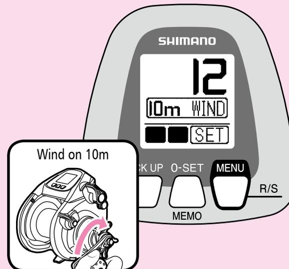
**6** Accurately wind on 10m of main line. The display changes in accordance with the number of spool revolutions.
