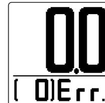
\* Do NOT wind or unwind the line when this Err error message is displayed. Line Learning will be inaccurate.
