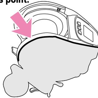
2. Remove the reel from the water and hold it up with the connector side facing down to ensure that the water completely drains from inside the reel.
