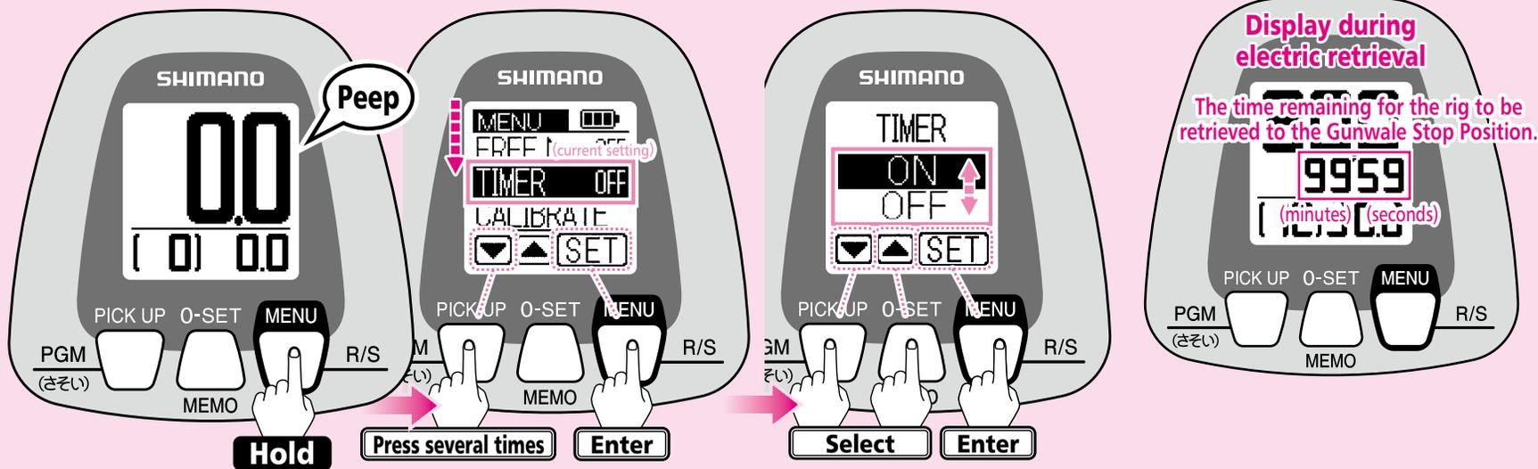
**1** When the power is turned on, Rig Retrieval Time is set to OFF. The illustration shows the Water Depth Display with Rig Retrieval Time OFF.
