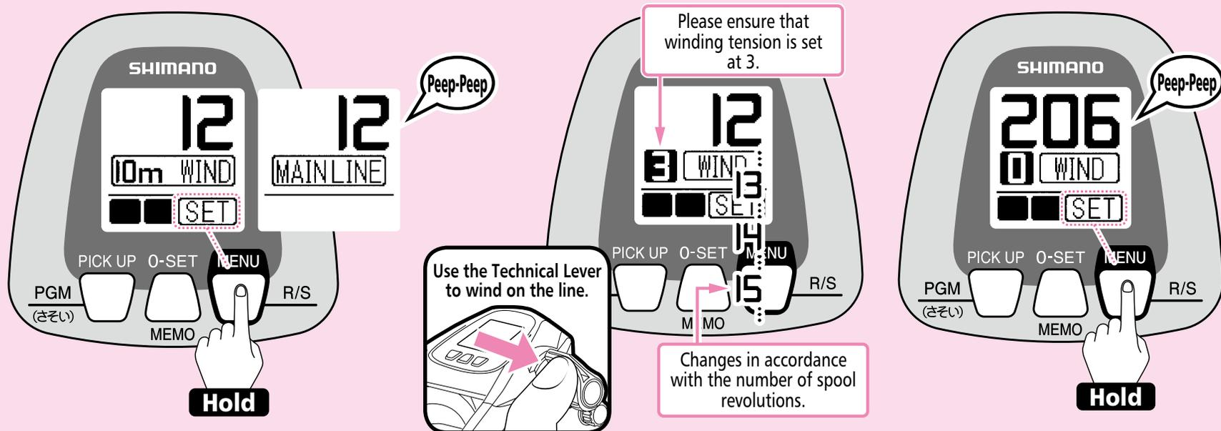
**7** Press the MENU button for more than 3 seconds. The alarm will sound (peep-peep) and the display will appear as shown in the diagram.
