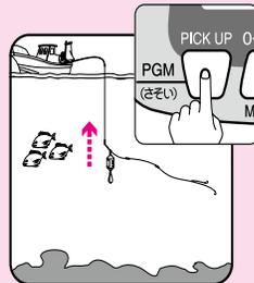
The motor winds in the line for as long as the button is pressed.
