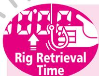
When retrieving the rig under power, this displays the time remaining for the rig to be retrieved to the Gunwale Stop Position.
